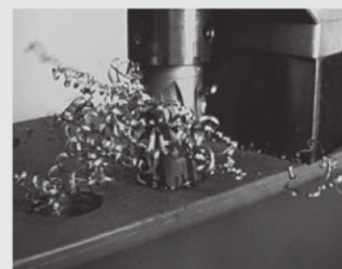
I-BEAM STEEL BORING
